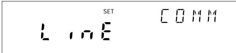
Communications display for setting the line frequency
