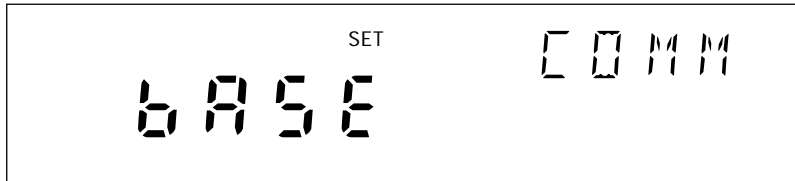
Communications display for setting the BCN
