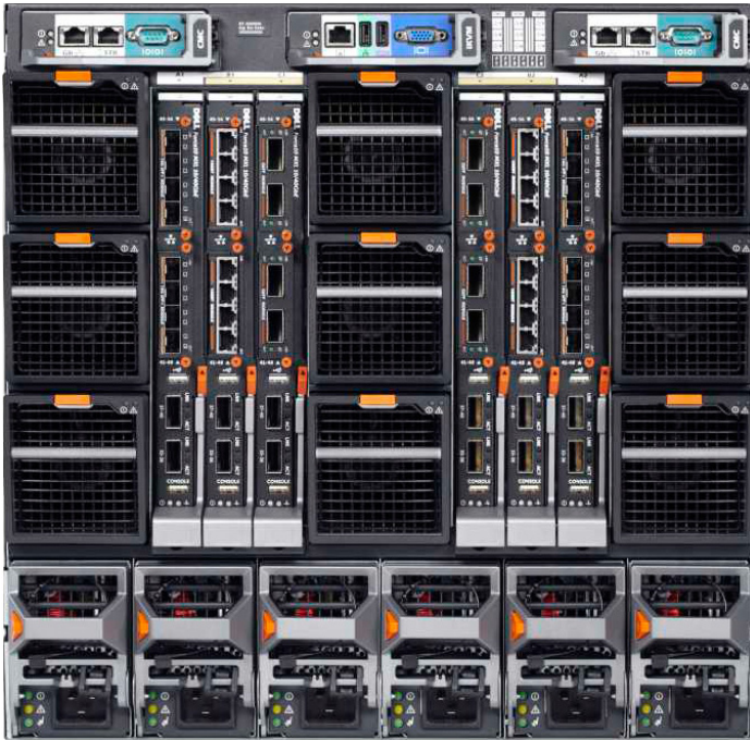
Figure 1-8. PowerEdge M1000e: Back View with Six MXL 10/40GbE Switch Blades
