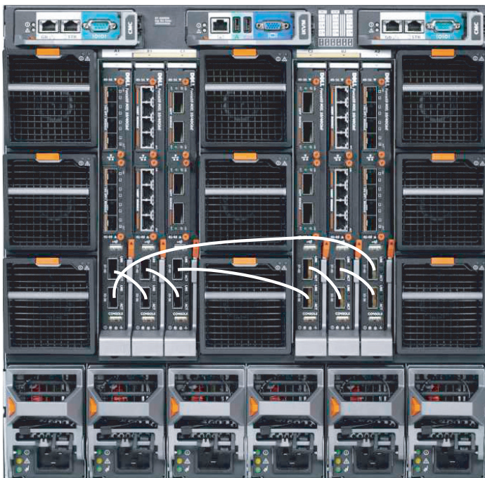
Figure 1-9. Six Stacked MXL 10/40GbE Switches
