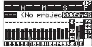
Input levels of channels 1 through 16 Stereo L and R buss output levels
