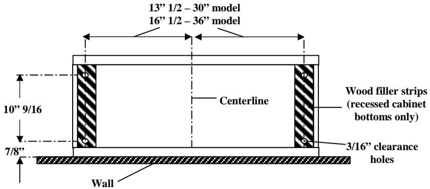
2. Add wood filler strips as needed to cabinet bottom. Drill four 3/16" clearance holes for hood mounting screws.
