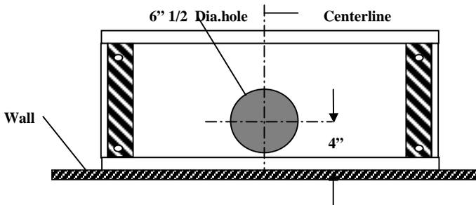
3. Cut 6 1/2" dia. hole in cabinet bottom as shown.
