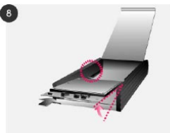
8 Insert the screwed HDD & PCB into a case of Freecom MediaPlayer-25 Drive-In Kit.
