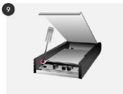
9 Screw HDD & PCB on the Freecom MediaPlayer-25 Drive-In Kit by using a screw driver.
