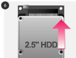
6 Grip HDD and insert it into the pins of PCB (be sure to match the 44 pins).
