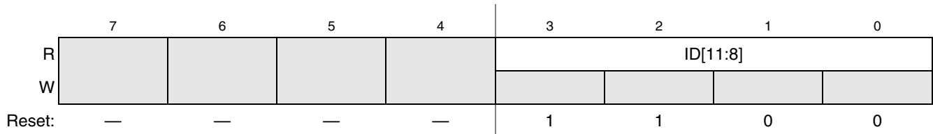
Figure 5-5. System Device Identification Register High (SDIDH)
