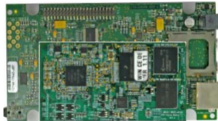
Figure 3.5 Install CPU Board onto Personality Board
