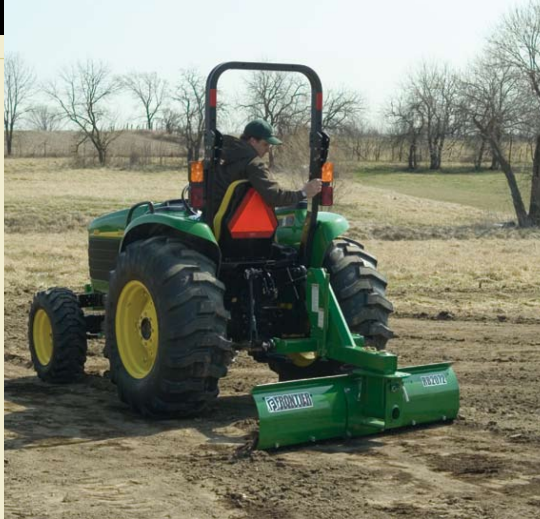
A formed, upper moldboard edge increases rigidity. Moldboard thickness is 3/16-inch for RB2060 and 1/4-inch for RB2072 and RB2084.
