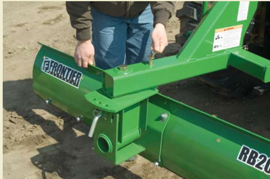
A formed, upper moldboard edge increases rigidity. Moldboard thickness is 3/16-inch for RB2060 and 1/4-inch for RB2072 and RB2084.
