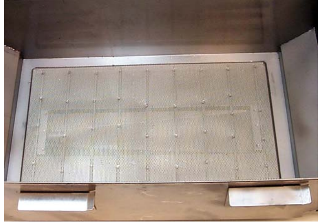
Support grid properly placed in filter pan.
