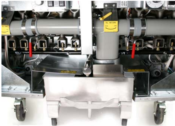
Typical Under Fryer Filter (UFF) installed in a multi-battered frying system.
