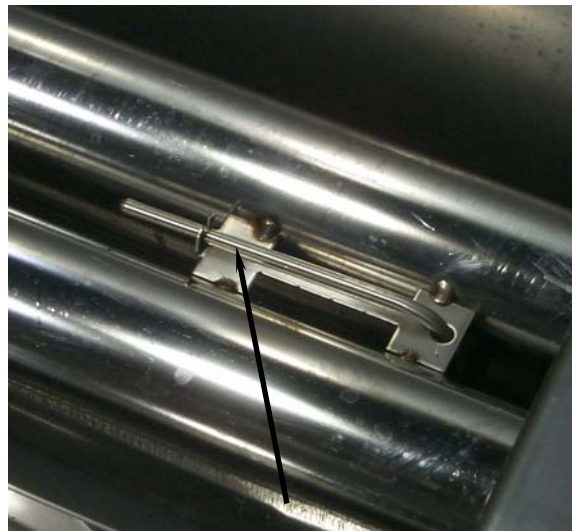
Electronic thermostat probe in frypot (arrow).
