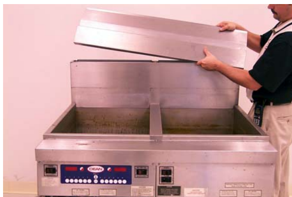
Removing the flue cap.
