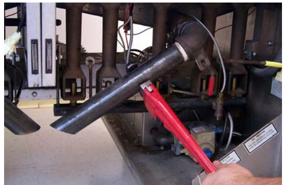
Removing 1.5" drain extension. (Step 19.A)
