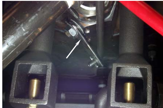
Remove cotter pin (arrow), then disconnect the actuator rod.
