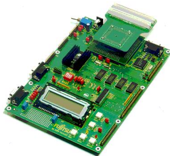
Figure 1: Using the Starterkit as target board for the ICE
