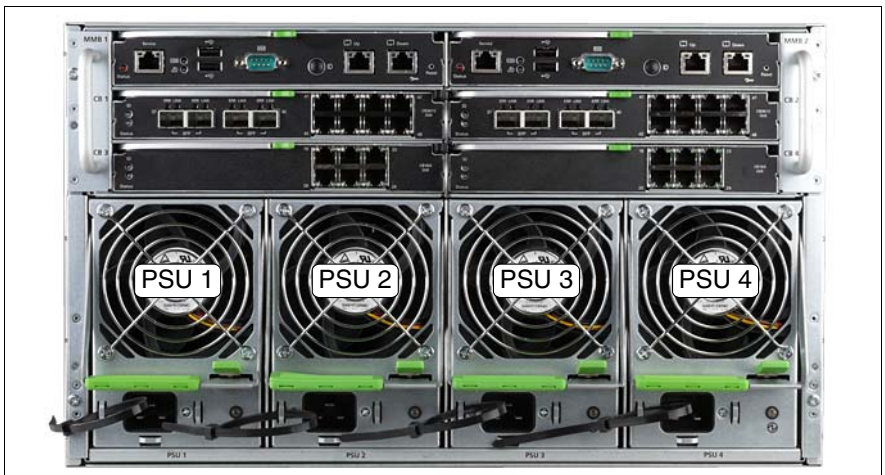
Figure 42: Numbering of the power supply unit bays
