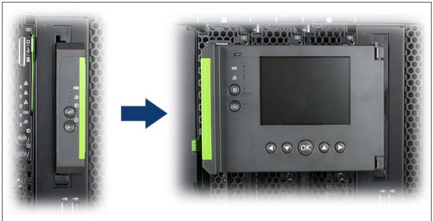
Figure 11: ServerView Local Service Display for Blade (rack version)
