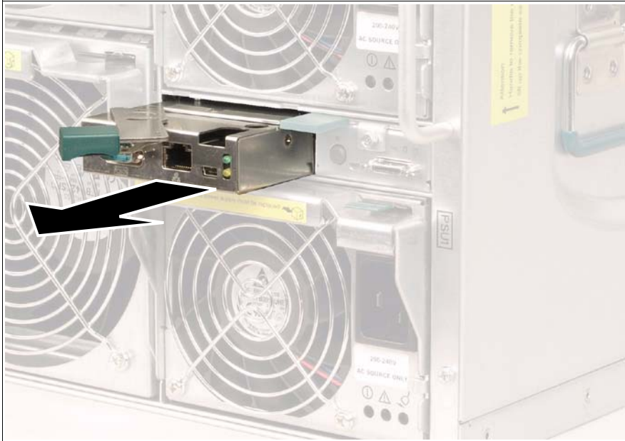
Figure 83: Removing the management blade
