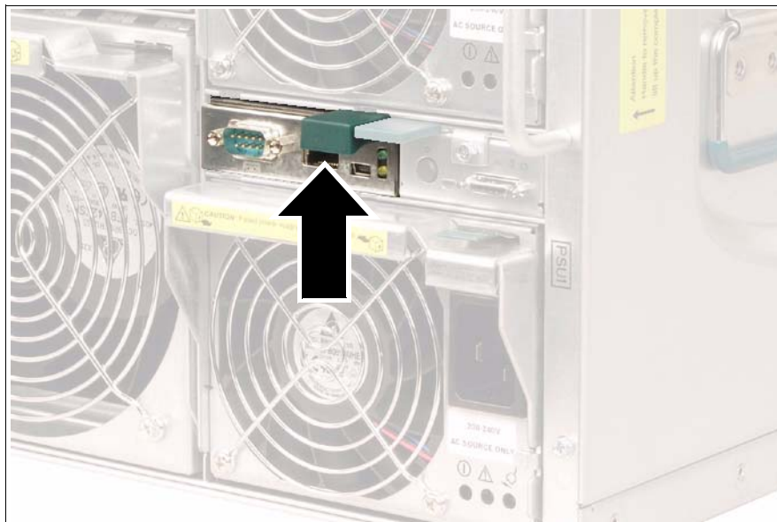
Figure 81: Disengaging the management blade
