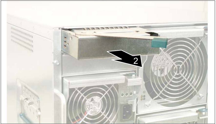
Figure 49: Removing the dummy module (a = green touch point)
