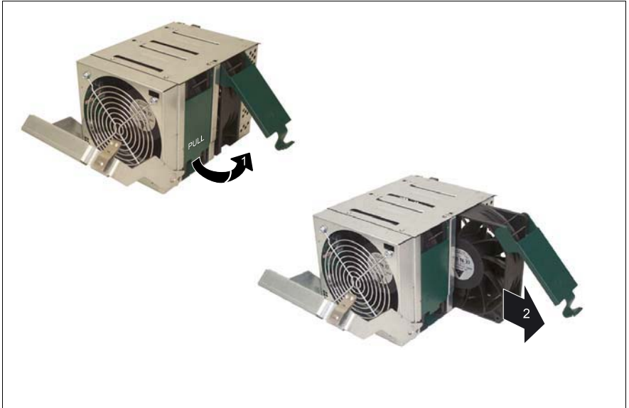
Figure 99: Disengaging the fan unit (a = green touch point)
