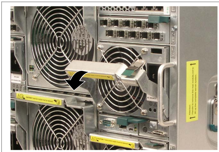
Figure 92: Removing the power supply unit
