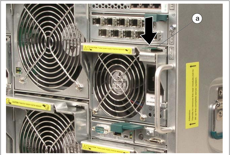
Figure 91: Disengaging the power supply unit (a = green touch point)
