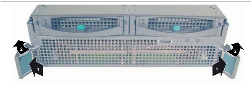
Figure 37: Turning the eject handles into the unlocked position (4-way server blade)
