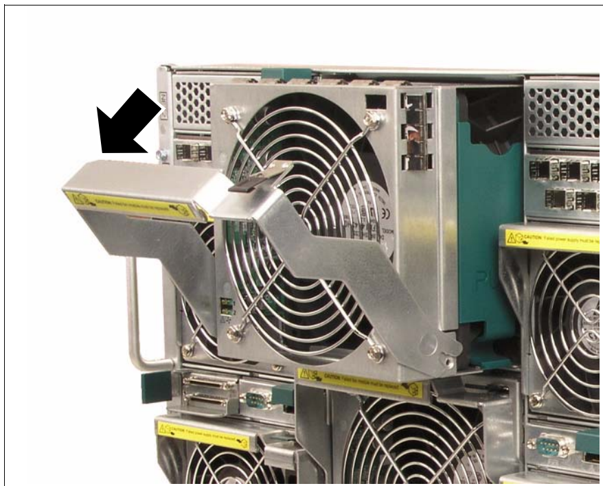
Figure 98: Removing the fan unit
