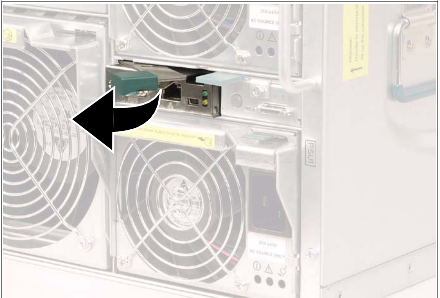
Figure 82: Disengaging the management blade
