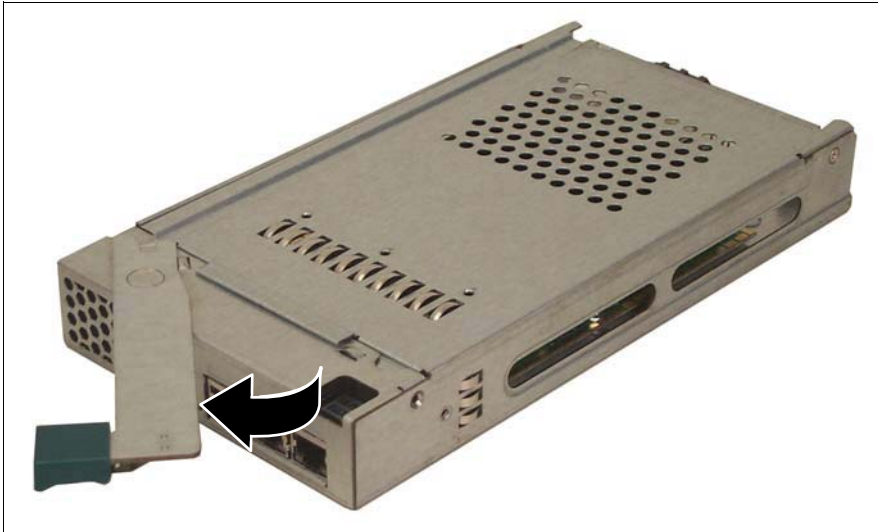
Figure 50: Disengaging the switch blade
