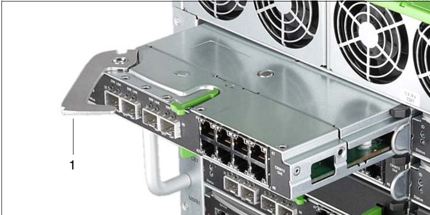
Figure 44: Installing a connection blade
