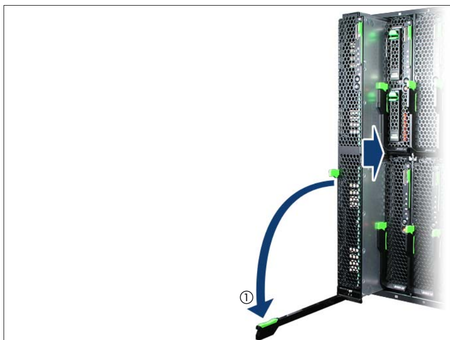
Figure 3: Installing the Server Blade
