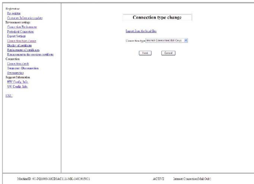
FIGURE 4.6 Window for changing the active connection configuration
