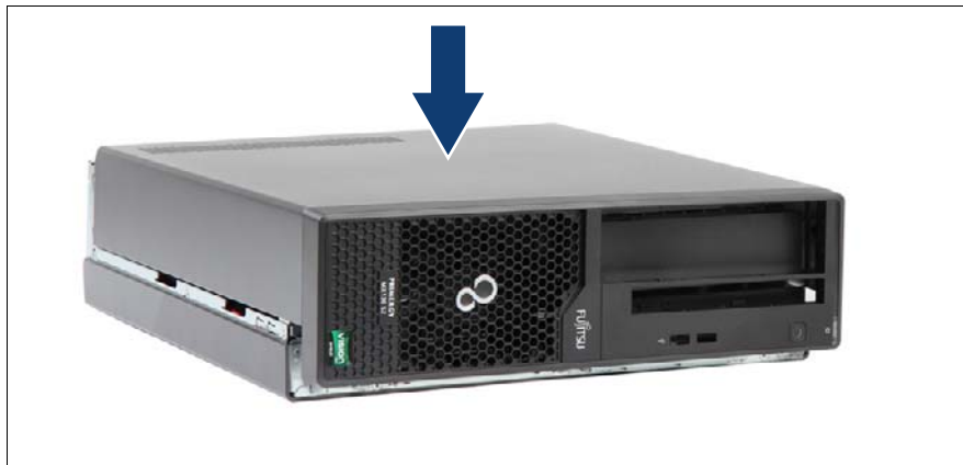
Figure 9: Mounting the server cover
