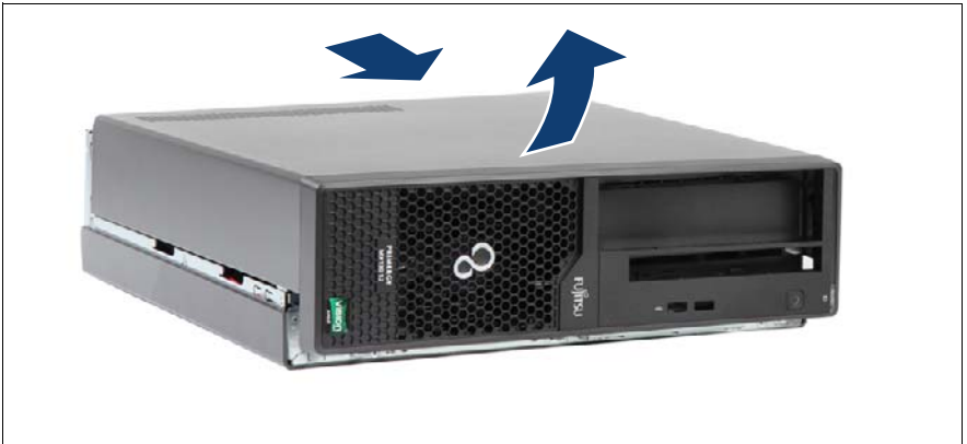
Figure 6: Removing the server cover
