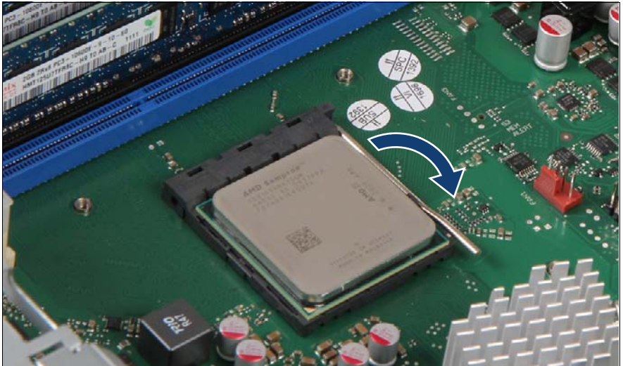
Figure 122: Latching the socket lever
