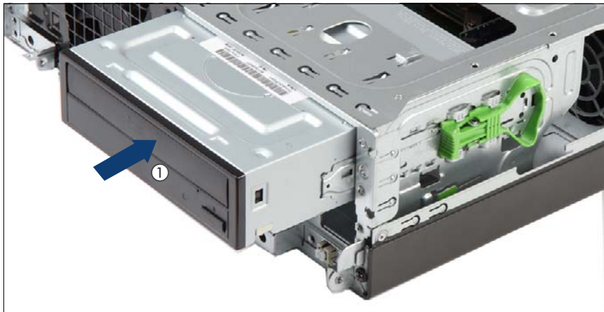
Figure 54: Installing HH ODD
