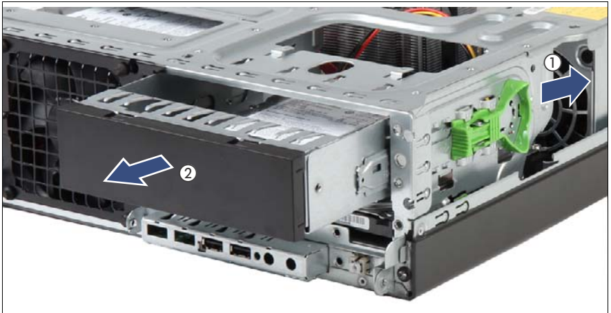
Figure 52: Removing the 5.25-inch dummy cover
