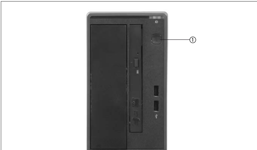
Figure 13: Power button on the front panel
