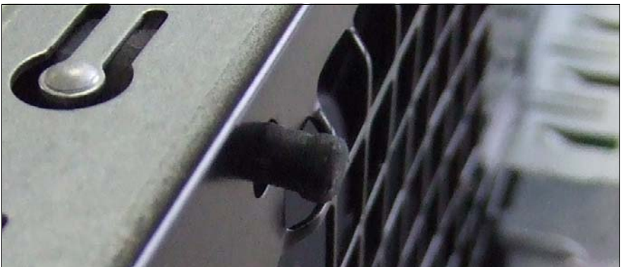
Figure 93: Initial position of a front fan rivet in the chassis fan slot
