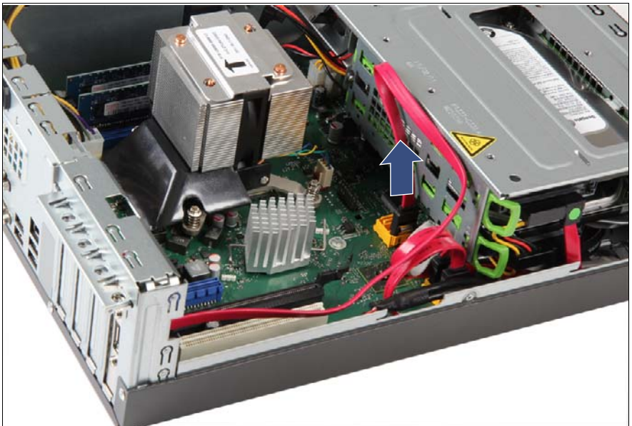
Figure 105: Disconnecting the eSATA cable
