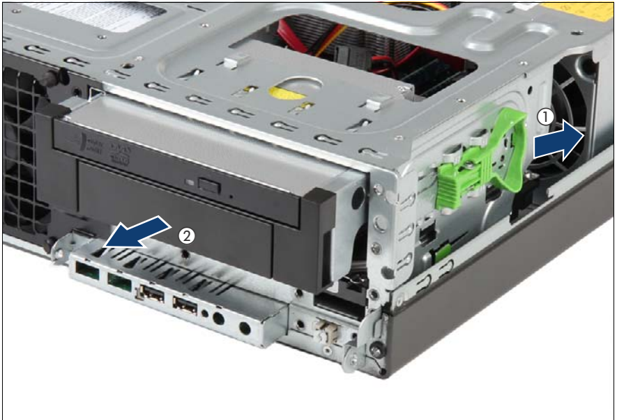
Figure 64: Removing the 5.25-inch ODD/HDD bracket with the slimline ODD
