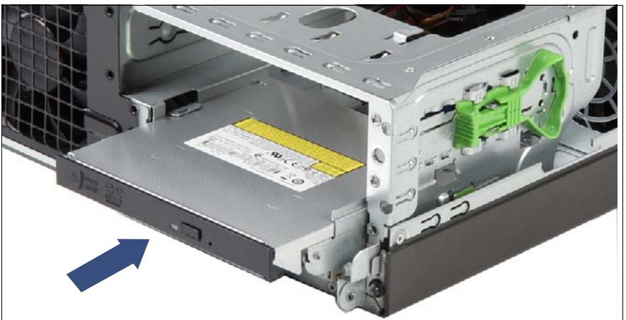
Figure 76: Installing the ODD
