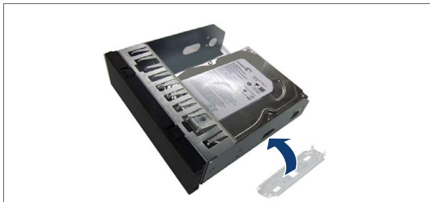
Figure 36: Connecting the fixation plate to the 5.25-inch dummy cover
