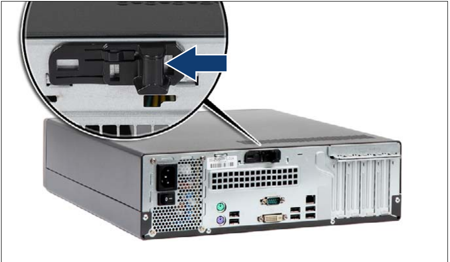
Figure 5: Unlocking the locking bar
