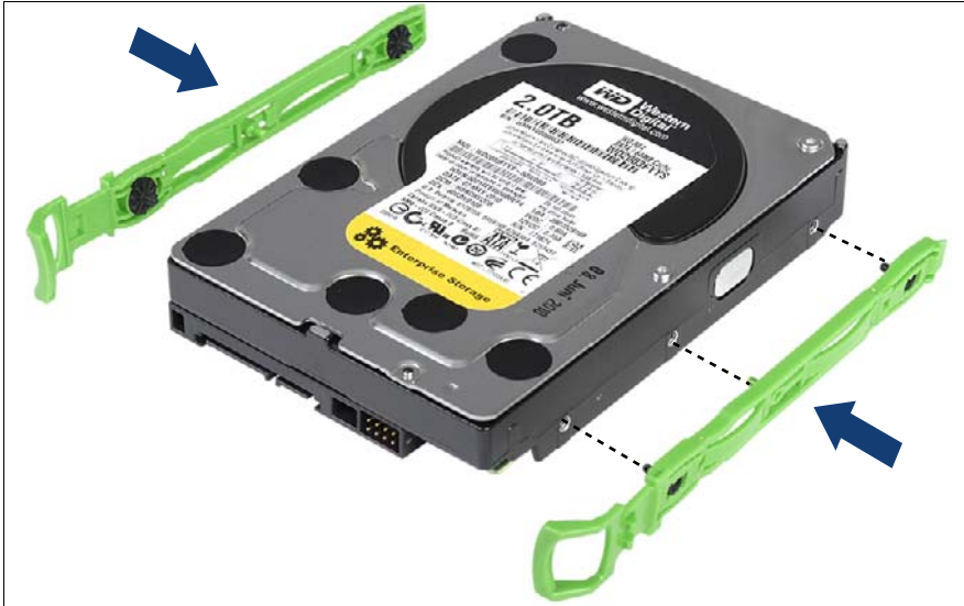
Figure 24: Installing the Easy rail on the 3.5-inch HDD
