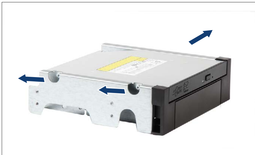
Figure 65: Removing the screws
