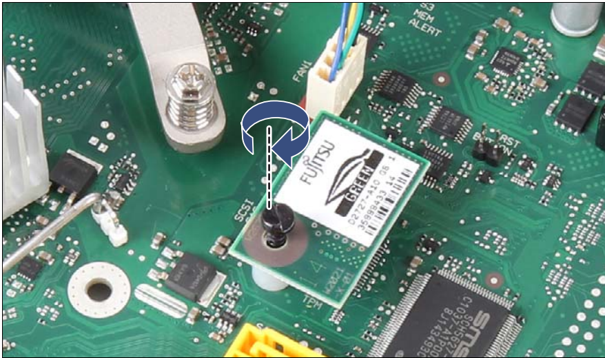
Figure 132: Securing the TPM board
