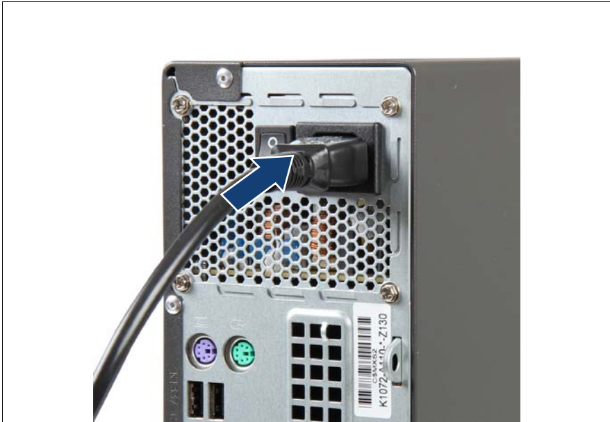
Figure 11: Connecting power cord
