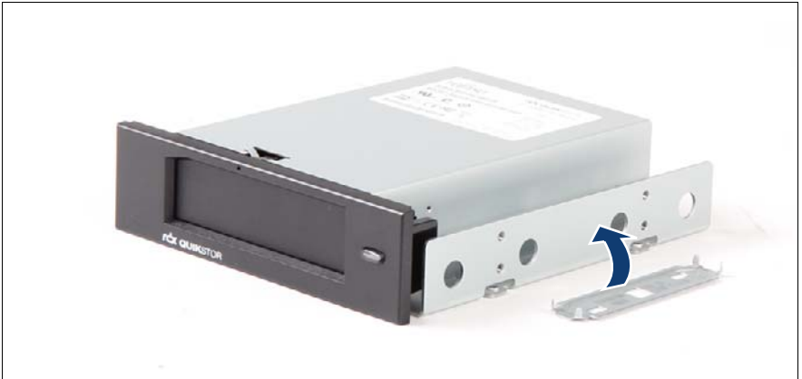
Figure 68: Connecting the fixation plate to the 5.25-inch chassis bay
