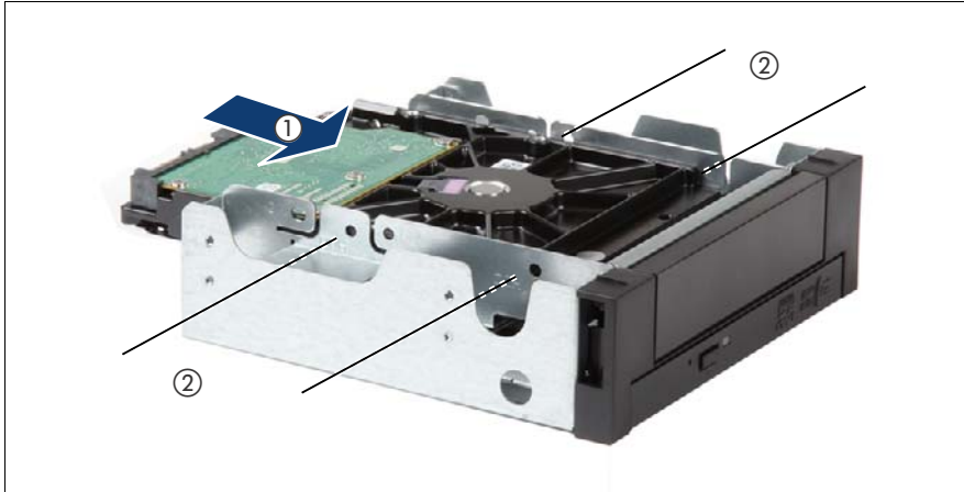
Figure 42: Installing the HDD in the 5.25-inch ODD/HDD bracket
