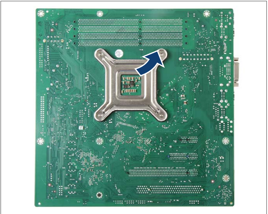
Figure 137: Removing the heat sink counter plate
