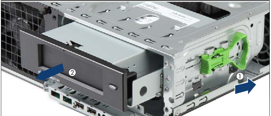
Figure 72: Removing the backup drive
