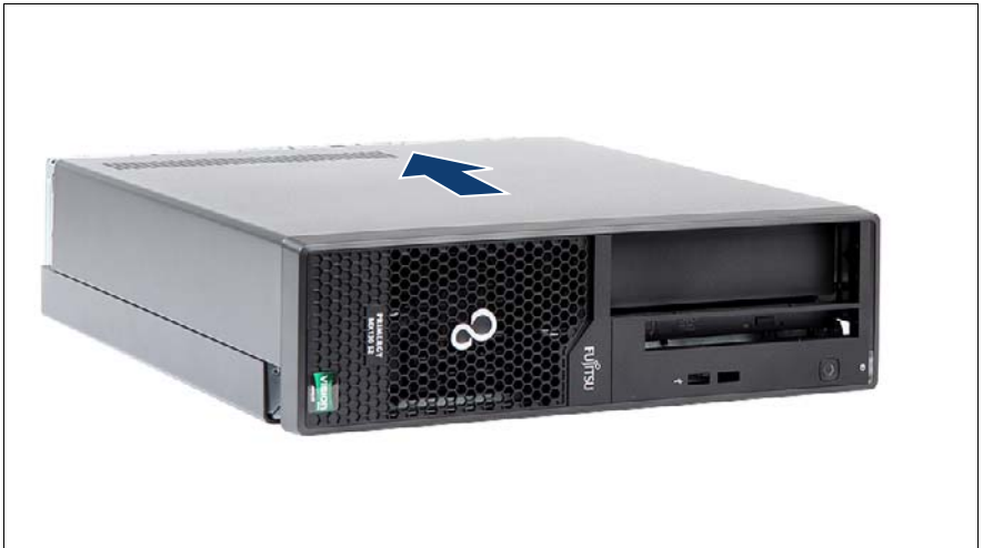
Figure 10: Closing the server cover
