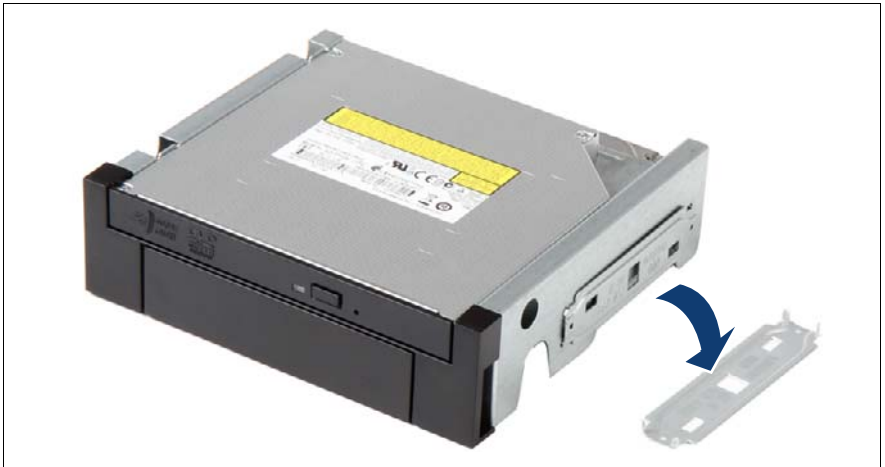
Figure 48: Removing the fixation plate from the 5.25-inch ODD/HDD bracket
