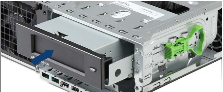
Figure 69: Installing the backup drive
