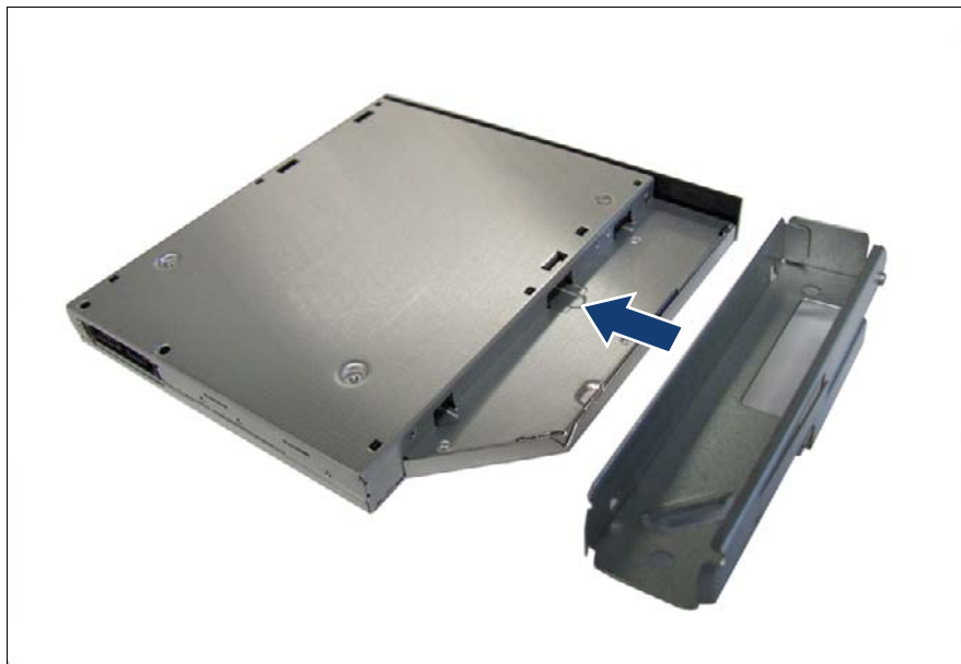
Figure 74: Installing the ODD
