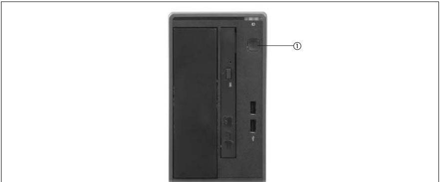
Figure 2: Power button on the front panel
