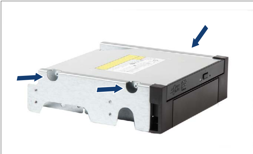
Figure 59: Fastening the screws
