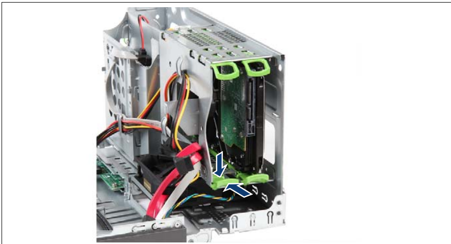
Figure 30: Inserting the Easy rails
