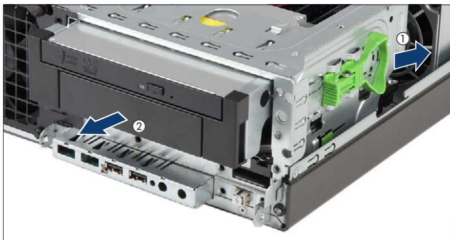
Figure 47: Removing the 5.25-inch ODD/HDD bracket
