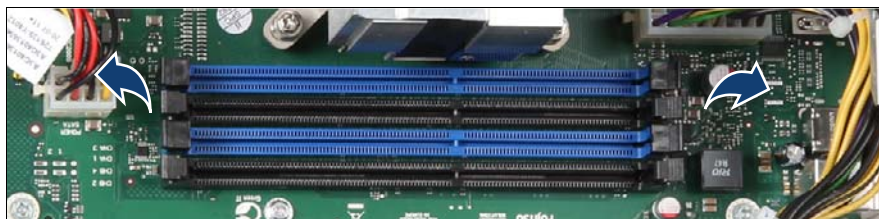
Figure 114: Installing memory modules (A)
