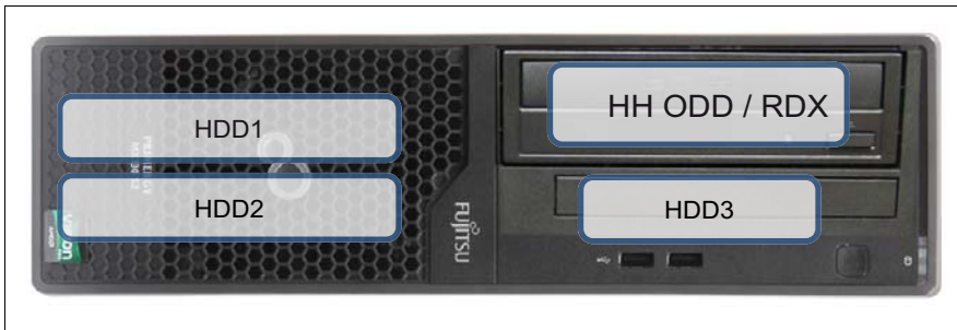
Figure 23: HH ODD or RDX mounting order with 3 x 3.5-inch HDD
