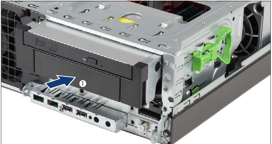
Figure 44: Inserting ODD/HDD bracket in 5.25-inch chassis bay
