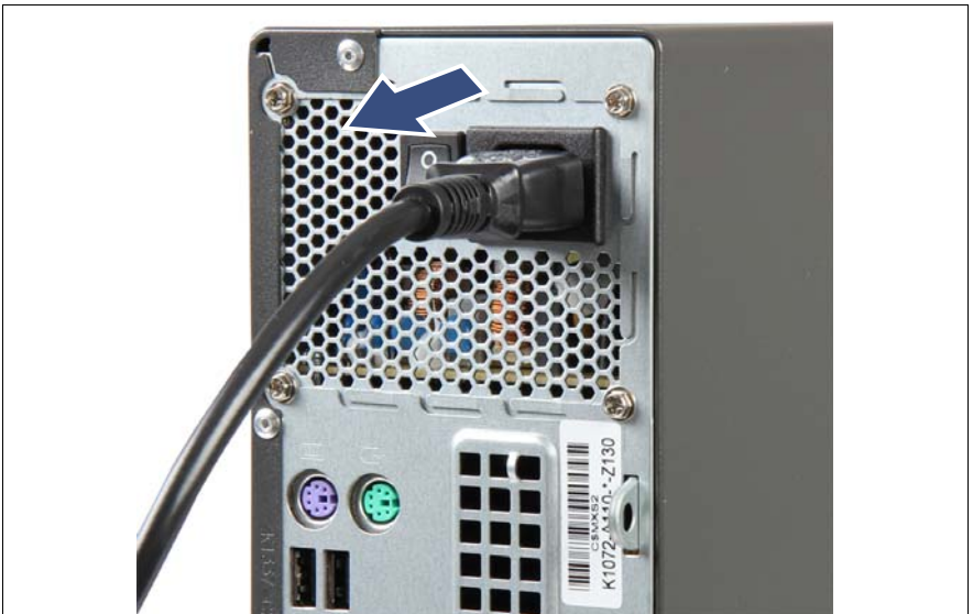
Figure 3: Removing the power cord from the PSU
