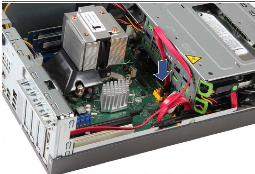
Figure 104: Connecting the eSATA cable
