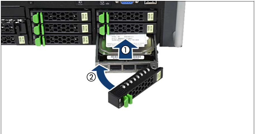
Figure 26: Installing the 2.5-inch HDD module
