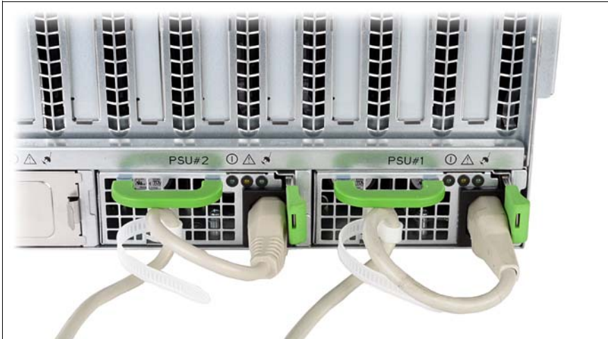
Figure 11: Cable clamps to secure the power cords
