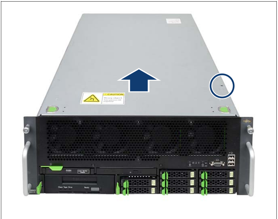
Figure 51: Opening the server
