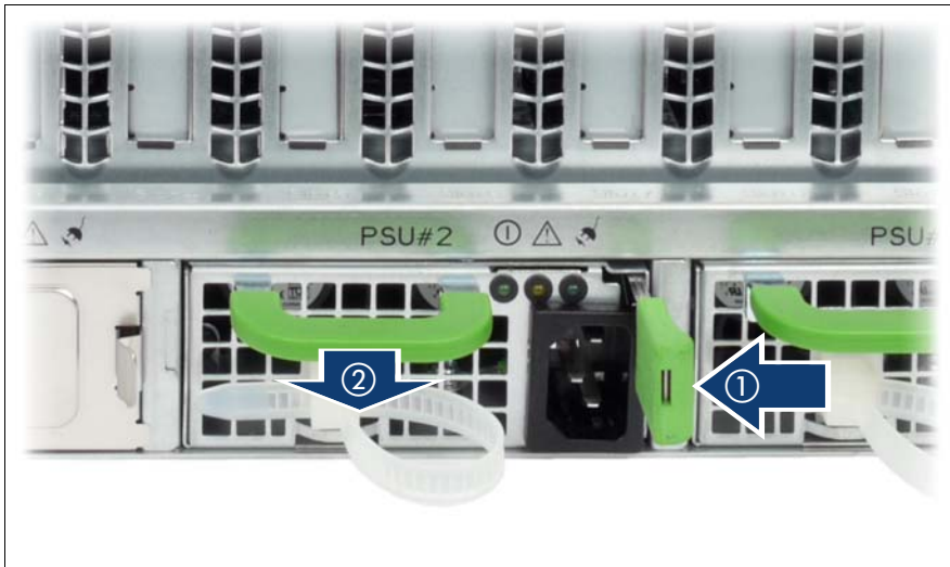
Figure 14: Unlocking and removing the power supply unit
