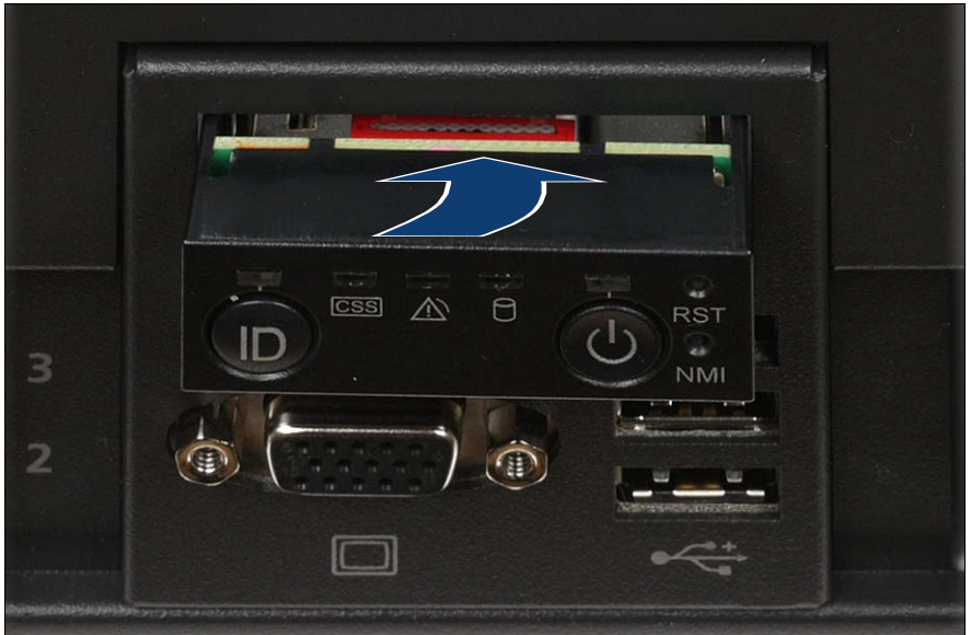
Figure 196: Installing the control panel
