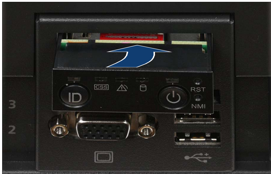
Figure 140: Installing the control panel
