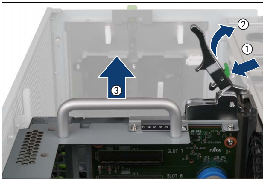
Figure 94: Removing the PCI Riser
