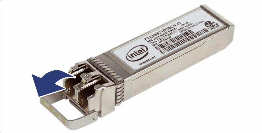
Figure 55: Unlatching the locking bail
