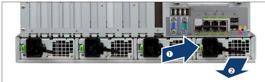
Figure 16: Unlocking and removing the power supply unit
