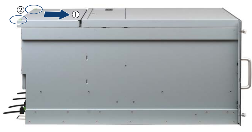
Figure 9: Installing the rear cover
