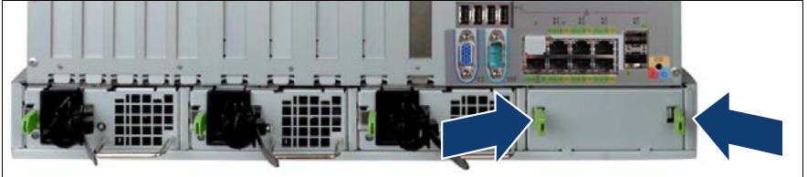
Figure 17: Installing a dummy module in a PSU bay
