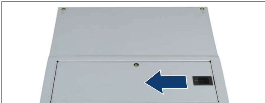
Figure 51: Closing the fan cover
