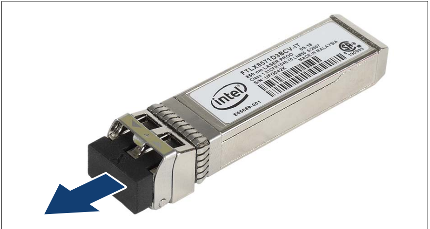
Figure 54: Removing the protective optical port plug
