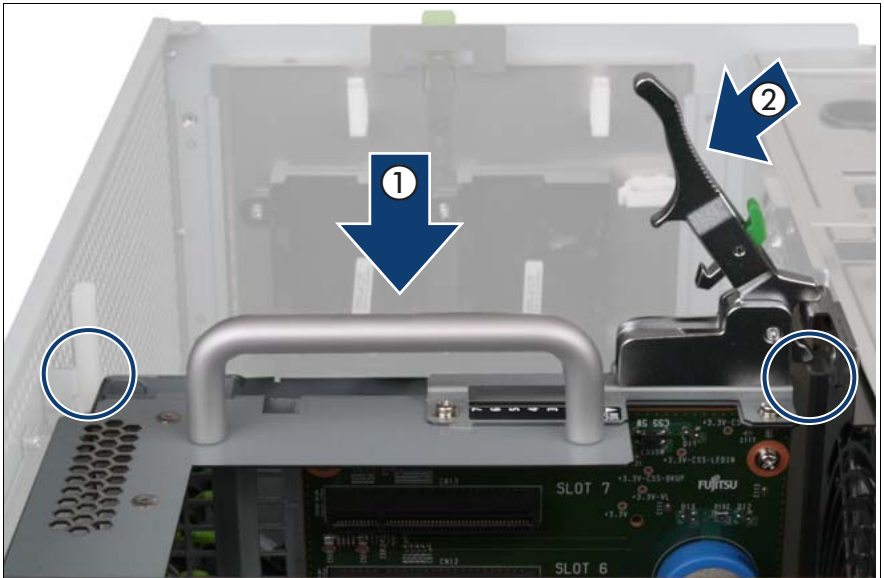
Figure 151: Installing the PCI Riser
