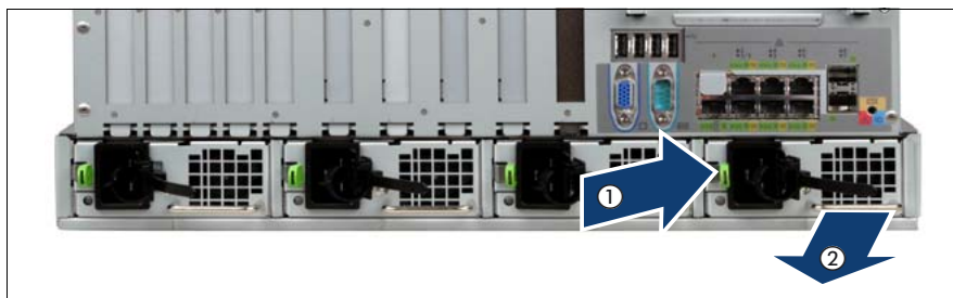
Figure 15: Unlocking and removing the power supply unit
