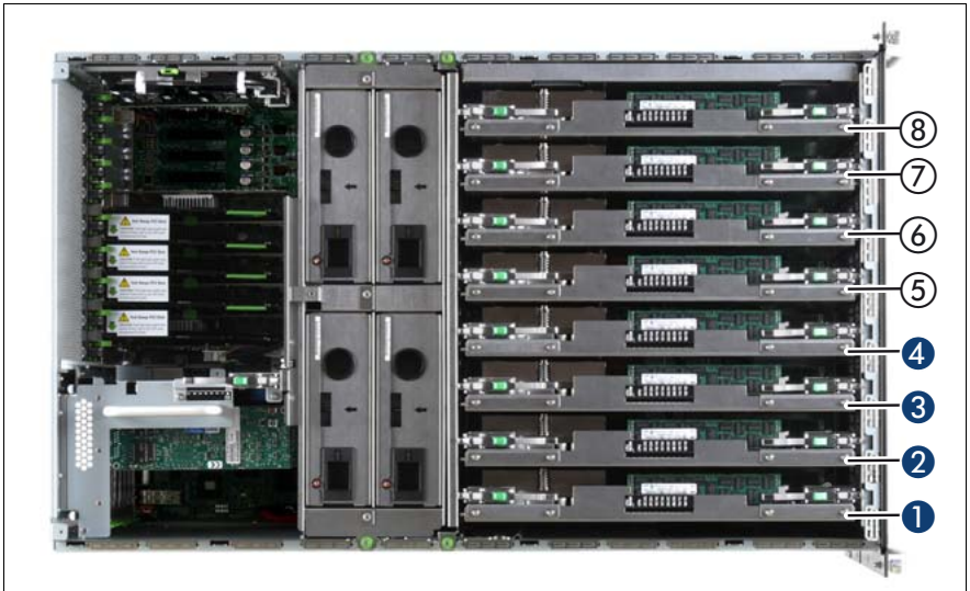
Figure 106: CPUMEMR slot assignment
