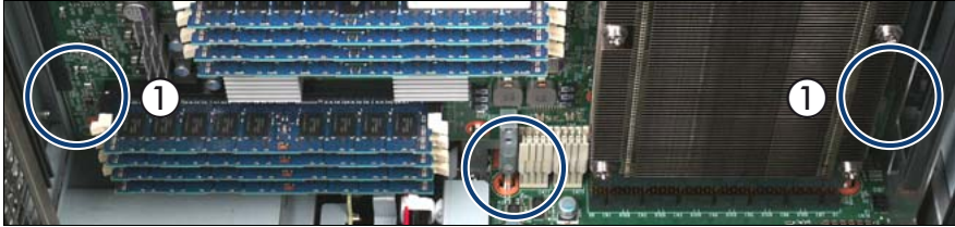
Figure 108: Inserting the CPUMEMR in the slot
