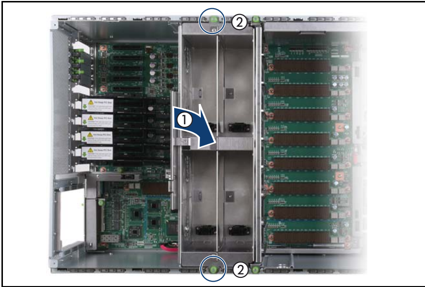
Figure 191: Inserting the fan cage
