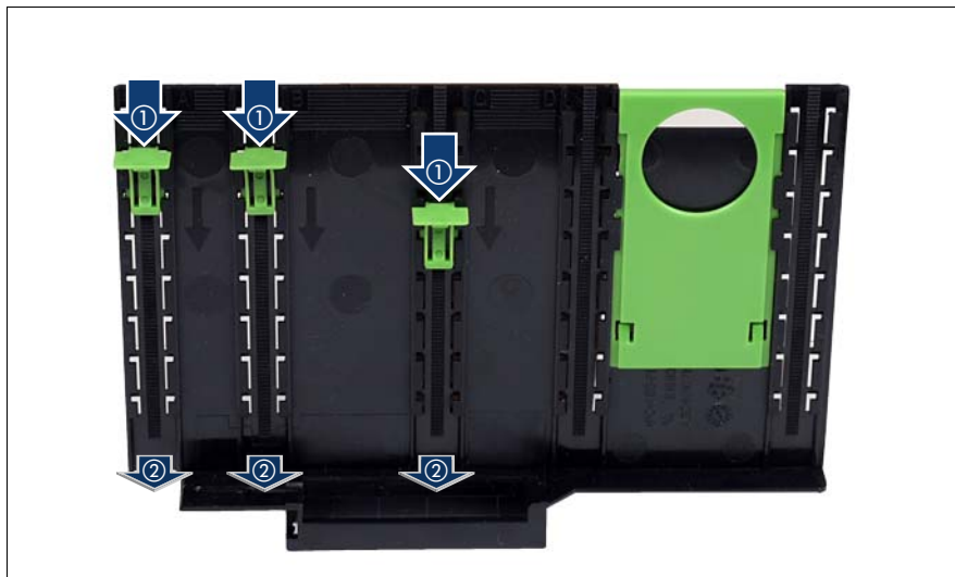
Figure 72: Removing the engaging hooks
