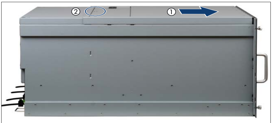
Figure 8: Installing the front cover
