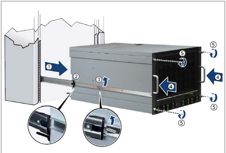
Figure 10: Inserting the server
