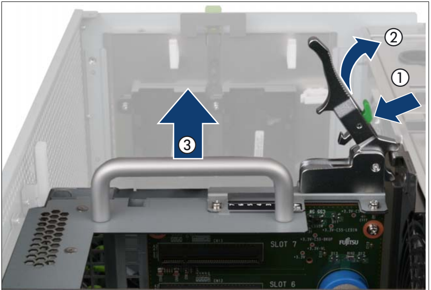
Figure 82: Removing the PCI Riser
