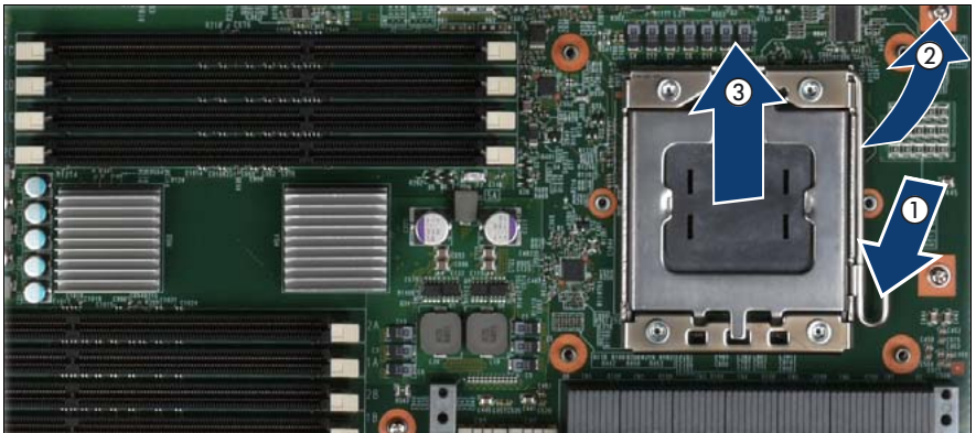
Figure 117: Removing the socket cover
