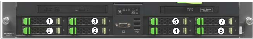
Figure 239: HDD/SSD bay numbering scheme
