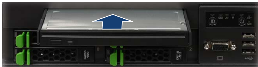
Figure 134: Sliding the optical drive in the bay
