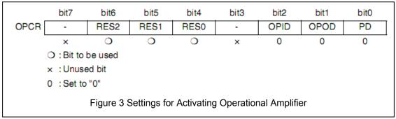
After the bits in the OPCR register are set as shown above, the operational amplifier will not start operating until it stabilizes.
