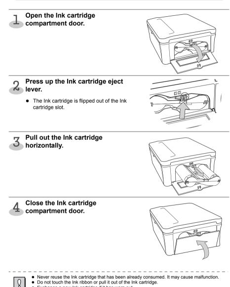
Exchange a new Ink cartridge if it has worn out.
