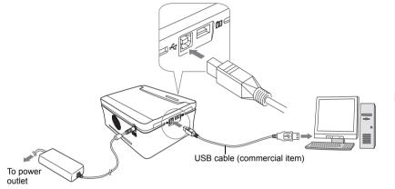
When connecting the printer to your computer, make sure that the connectors on the ends of the USB cable match the ports on the printer and on your computer. For the location and the terminal form of the USB port on your computer, refer to the user's guide of your computer.
