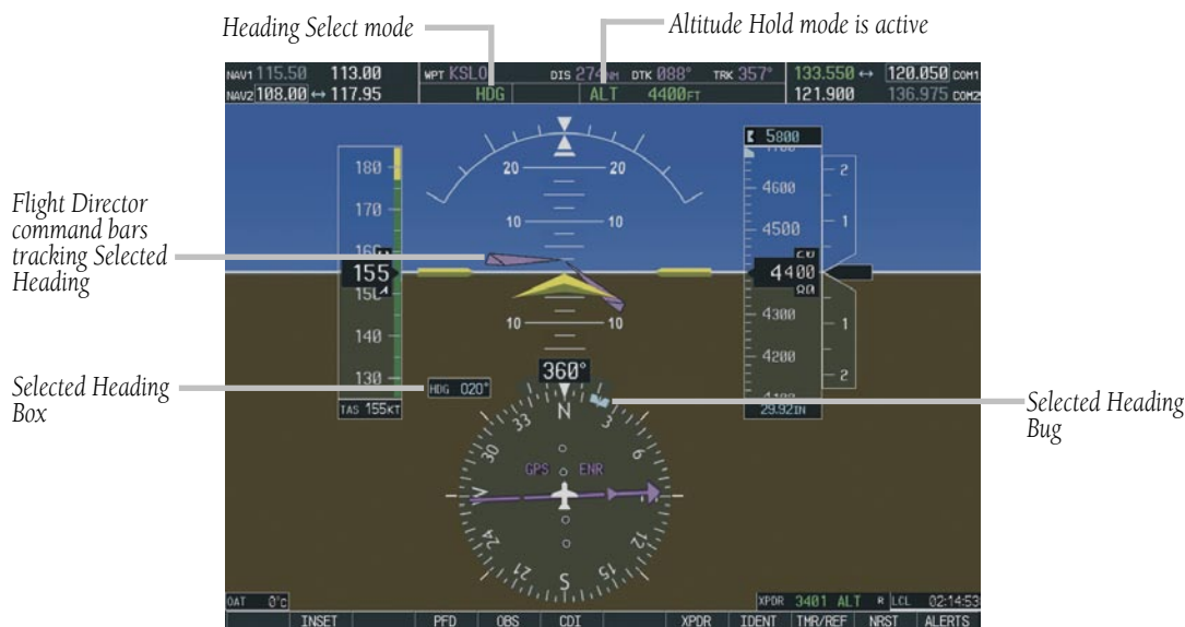
Figure 6-16 Heading Select Mode
