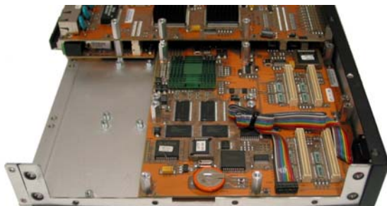
Figure 3.5.1c: Magnum 6K32F Series modular slot side (front-right side), without chassis cover
