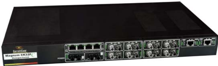
Figure 2.2.1a: A typical 6K32FC Switch front view, 4 RJ-45 10/100 ports, 2 ST 10Mb FL ports, 8 ST 100Mb FX ports and 2 RJ45 Gigabit ports.
