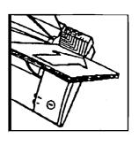
2a. Plug in and switch on 250T. BOOK PREPARATION 3. Firmly hold sheets to be bound and place binding edge on lined surface. The first horizontal line above the paper will indicate the cover size to use.
