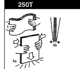
4a. Fan and jog paper to insure that all edges are even. 4b. Before inserting pages into binder, square the spine along the 2 inside score lines.
