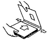
5. Holding sheets firmly, insert fully into cover until they are all directly and evenly seated against the spine adhesive.
