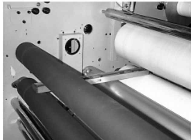
Figure 2-7: Leveling Front to Rear
