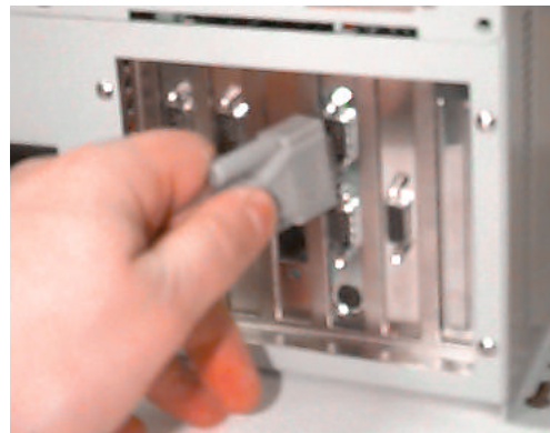
Figure 11. Connecting a dumb terminal to the RS232 port.
