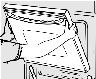
Lift the door straight up and off the hinges.
