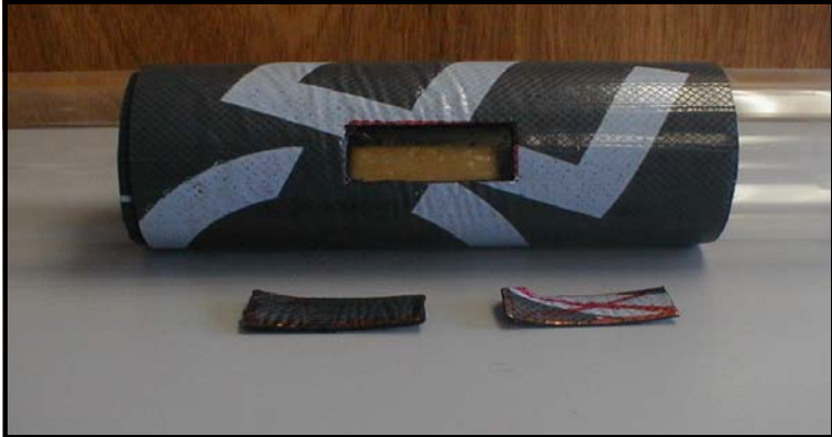
Figure 3-25: DMP-1 Material with Transducer Footprint Cut Out
