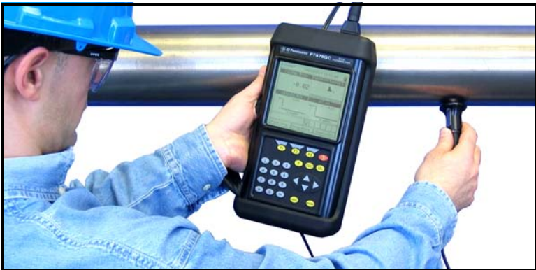
Figure 9-4: PT878GC Thickness Gauge in Operation
