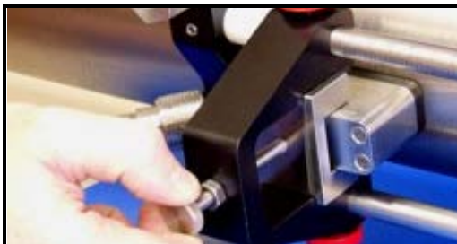
Figure 3-11: Installing the First Transducer
