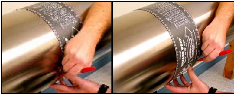
Figure 3-13: Marking Circumferential Lines on the Pipe
