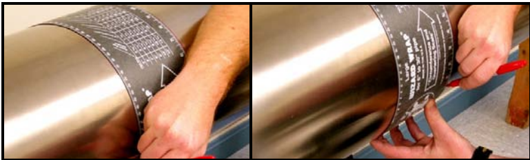
Figure 3-5: Measuring and Marking Circumference Lines
