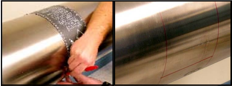
Figure 3-14: Marking the 3 o'Clock Position
