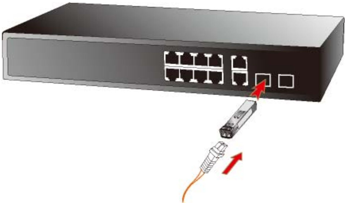
Figure 8: Plugging-in the SFP transceiver
