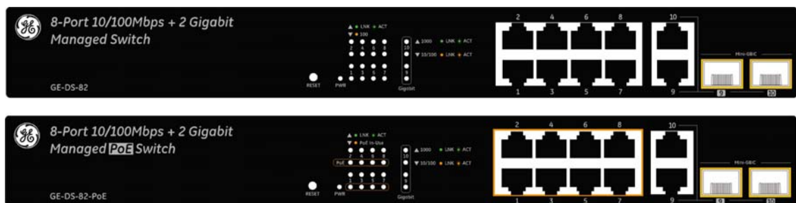
Figure 1: GE-DS-82 and GE-DS-82-PoE Switch front panels
