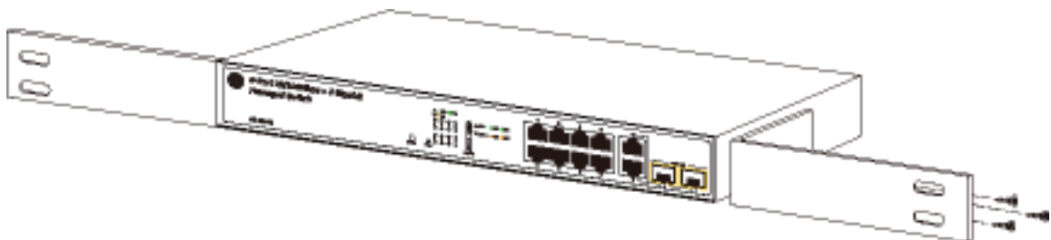
Figure 6: Attaching rack-mount brackets to the GE-DS-82
