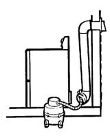
Inspect and clean the dryer exhaust ducting at least once a year to prevent clogging. A partially clogged exhaust can lengthen the drying time. To clean the exhaust duct follow these steps:
