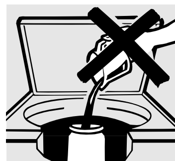
Do not pour anything into the agitator if the top is removed
