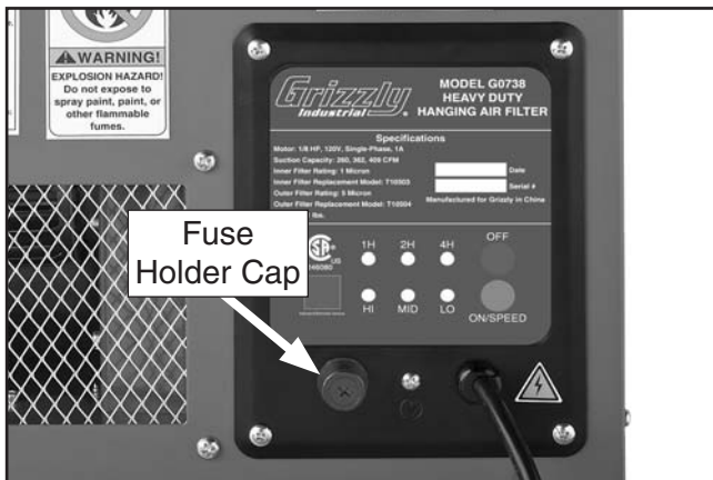
Figure 16. Fuse holder cap on the control panel.
