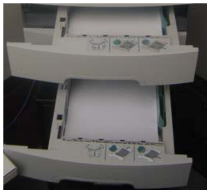
Paper tray with sloped front and no paper gripping corners
