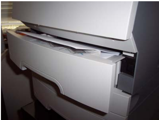
Excess paper being pushed out after overfilling
