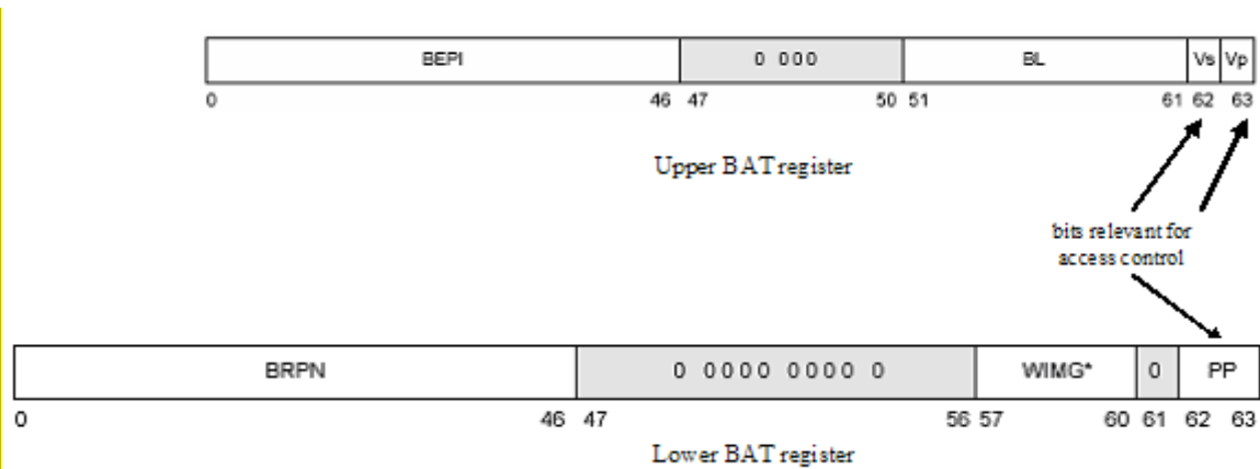
Figure 5-45: Block Address Translation entry
