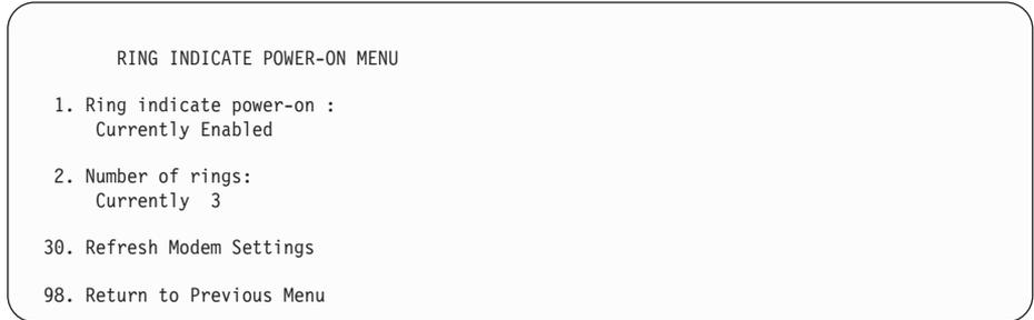
Ring indicate power-on is enabled by default on both serial port 1 (S1) and serial port 2 (S2). When ring indicate power-on is enabled, call-in is disabled.
