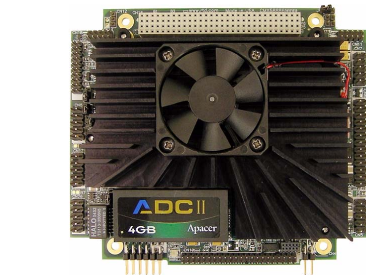
Figure 5 CMX158886 before and after ATA/IDE Disk Chip Installation
