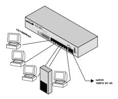
Computers are connected via copper cabling.
