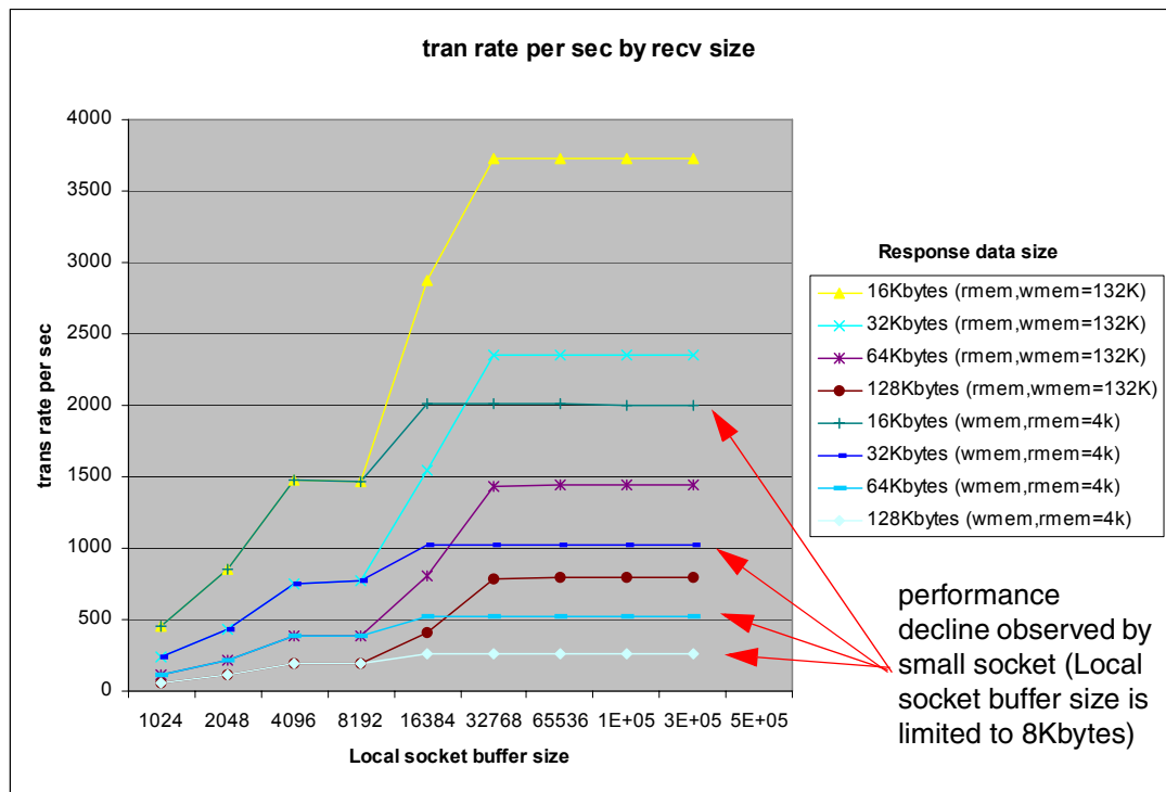
Figure 4-16 the comparison with socket buffer 4Kbytes and 132 bytes
