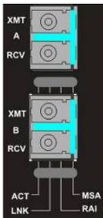
One model offers two *SFP* (A and B) ports for 1+1 protection; a second model offers one *SFP* without protection.
