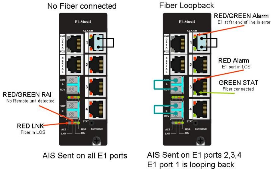
By placing a physical loopback connection on the E1 port, a valid signal can be detected by each individual E1 port to verify its operation. Without the fiber looped, the ALARM LED for the looped E1 port will show RED/GREEN indicating there is a problem at the far end of the fiber transport (In this case the far end unit is missing) and the STAT LED is RED because the fiber is in LOS. With the fiber looped, the E1 port will only show a normal GREEN STAT LED.
