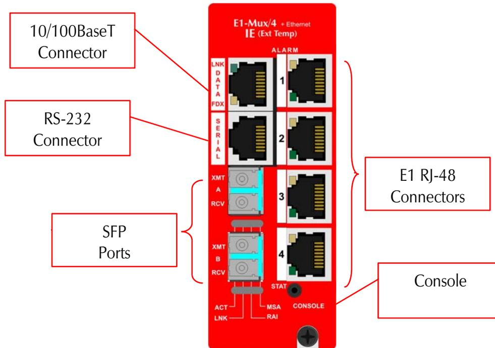
The IE-iMcV-E1-Mux/4 includes a console serial port. To establish a link between a module's console port and a local PC, connect the Mini Jack to DB9 adapter that is included with the IMC module. This RS-232 serial connection provides access to the IE-iMcV-E1-Mux/4 module *CLI* configuration screens. Set the computer/terminal for **VT-100 emulation, 38.4K baud, 8 data bits, 1 stop bit, no parity and no flow control**. Under the VT-100 emulation, set the backspace key to send delete.
