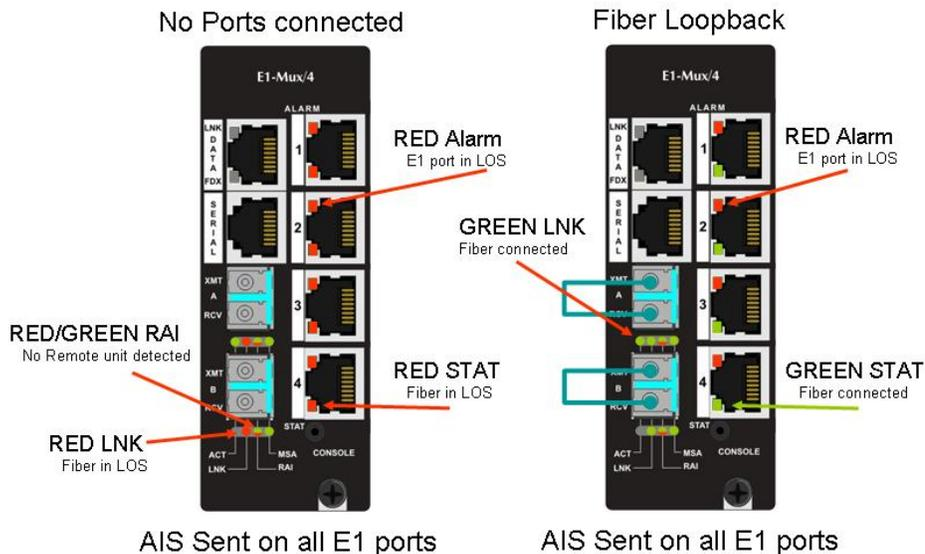
The *ACT LED* will arbitrarily be configured to either the A or B fiber line. The *RAI LED* is RED/GREEN indicating that there is something wrong at the far end of the fiber line (in this case, the remote unit is missing). The *ALARM LED* is RED because the E1 port is not connected. The *STAT LED* is RED when there is no fiber link but turns GREEN when the fiber link is valid.
