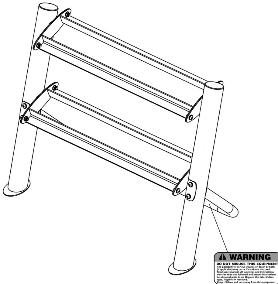
The Warning Label shown here has been placed on the Stabilizer. If the label is missing or illegible, please call customer service at 1-800-999-8899 for replacement. Apply the label in location shown.
