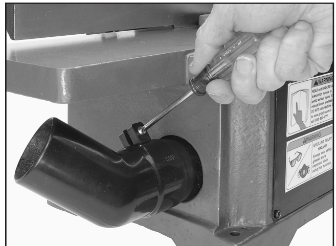
Figure 19. Installing the dust chute.
