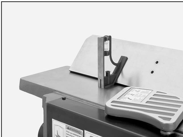
Figure 27. Checking the outward 45° stop.
