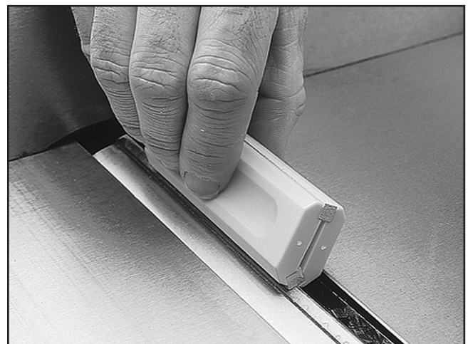
Figure 41. G3631 Jointer/Planer Knife Hone.
