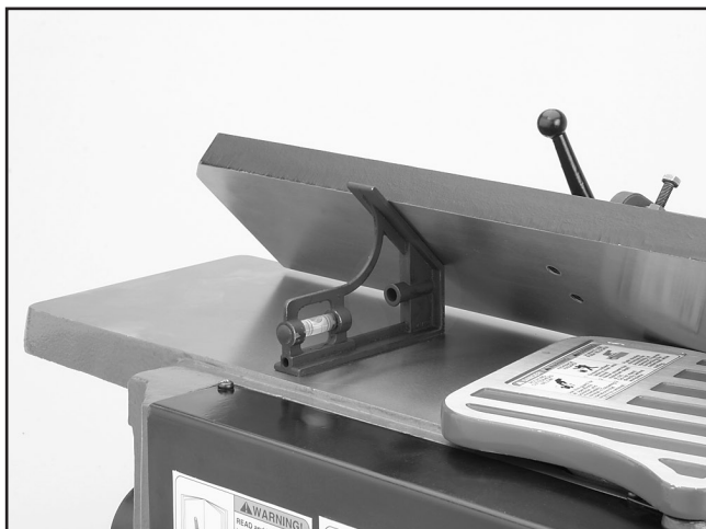
Figure 25. Checking the inward 45° stop.
