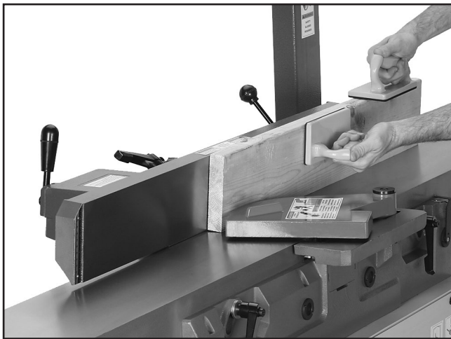
Figure 34. Typical edge jointing operation.
