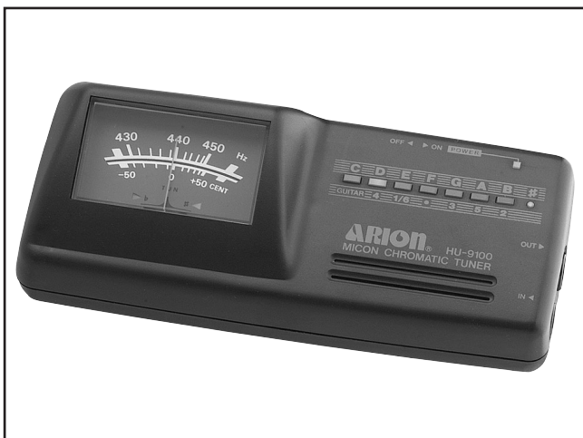
Figure 35. Model H3097 Chromatic Tuner.
