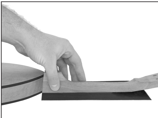
Figure 14. Flattening the neck.
