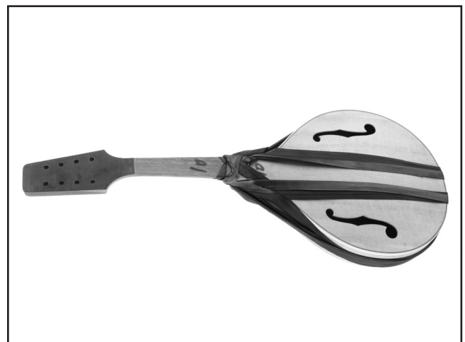
Figure 13. Example of gluing the neck.
