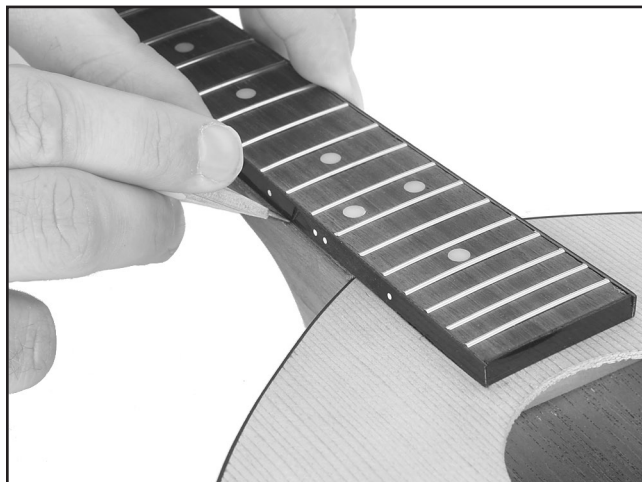
Figure 10. Marking fretboard binding edges onto neck.
