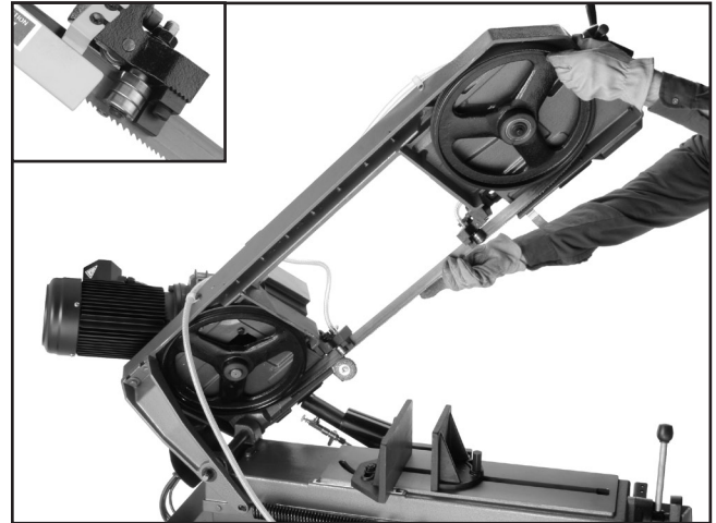
Figure 39. Typical blade installation.
