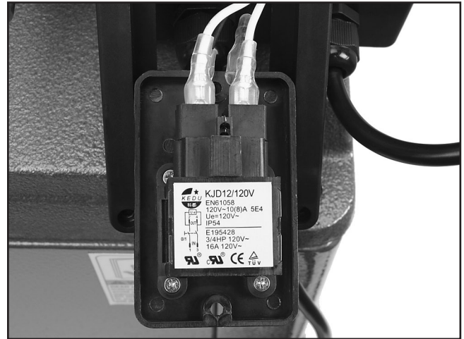
Figure 43. Switch wiring rear view.
