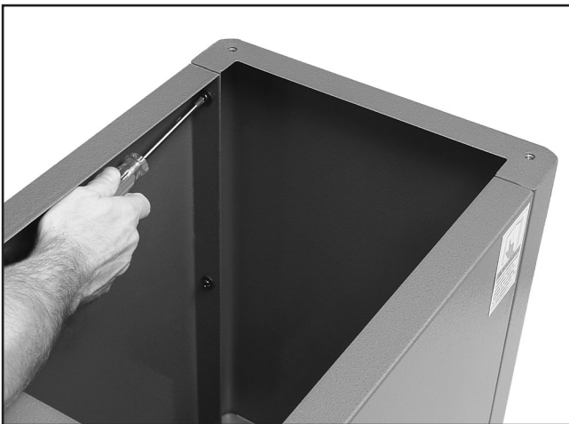
Figure 9. Installing right panel.
