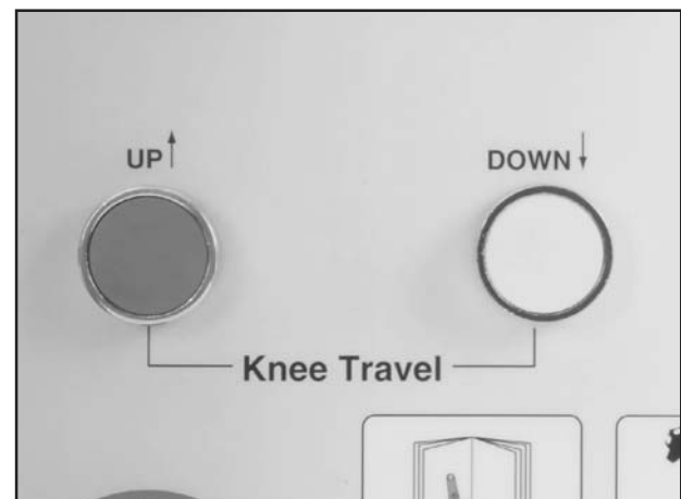
Figure 40. Z-axis (knee) power feed controls.
