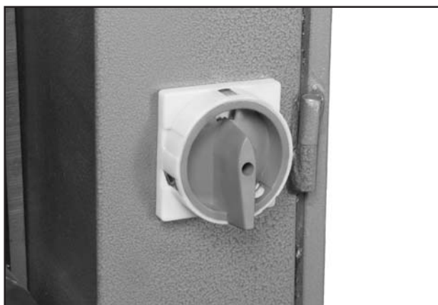
Figure 18. Main power switch in the OFF position (Model G0615 shown).
