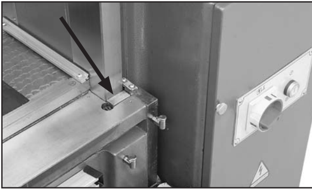
Figure 85. Model G0616 column gib and adjusting screw (shown from right top of knee way).
