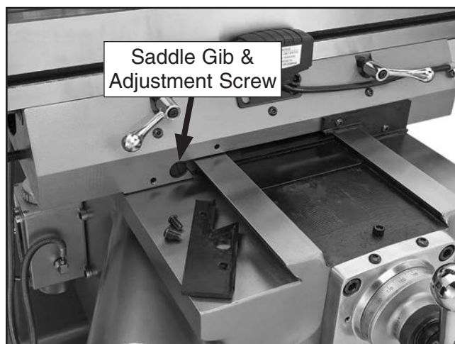
Figure 63. Saddle gib and adjustment screw.
