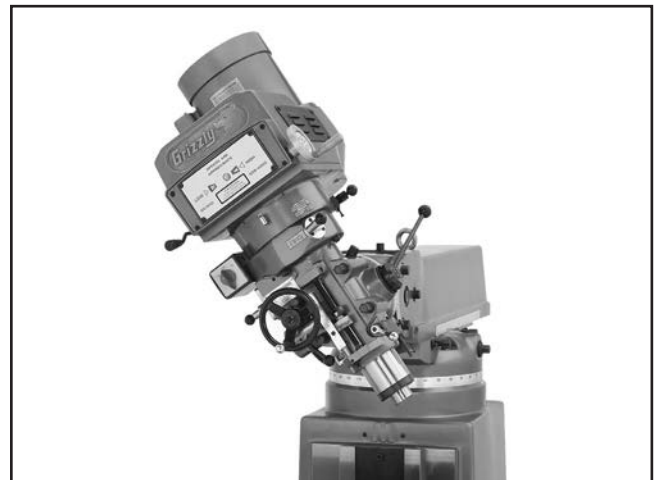
Figure 21. Head rotated to the left.
