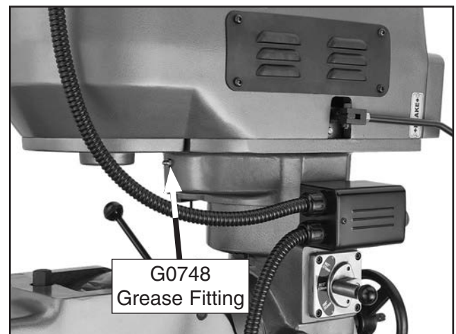
Figure 55. Model G0748 headstock gearing grease fitting.
