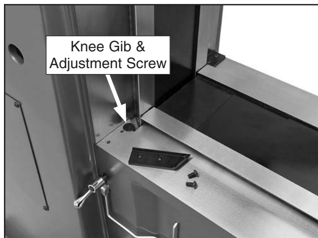
Figure 64. Knee gib and adjustment screw.
