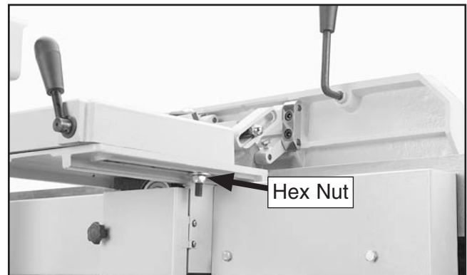
Figure 15. Fence installed on mounting bracket.
