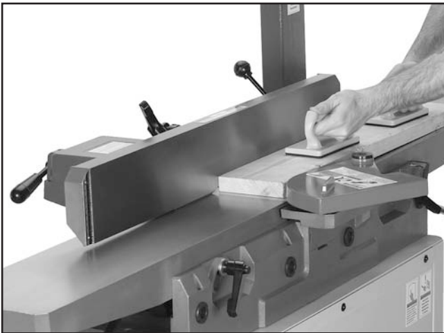
Figure 25. Example of surface planing with the jointer.
