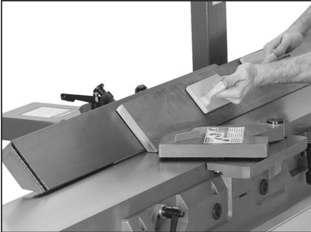
Figure 29. Fence setup for a bevel cut of 45°.
