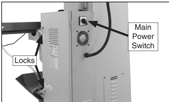
Figure 21. Main power switch on back of electrical cabinet.
