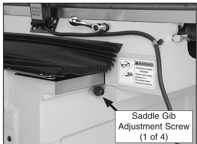
Figure 63. Saddle gib adjustment screw (view of right front screw).
