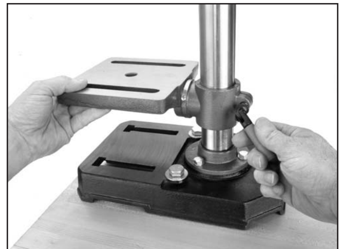
Figure 10. Securing table support.
