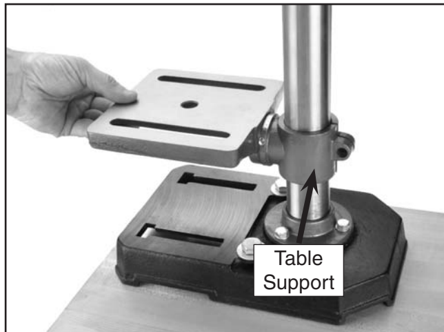
Figure 8. Installing table support.
