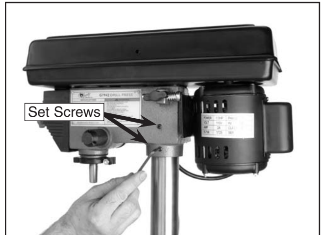
Figure 11. Securing headstock with set screws.
