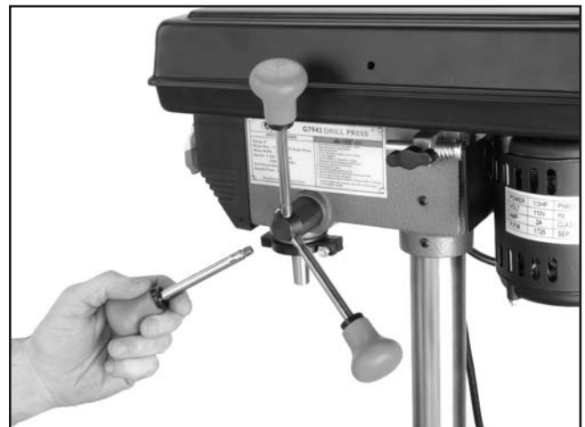
Figure 12. Installing feed handle.
