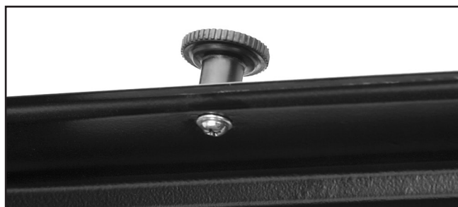
Figure 9. Knob installed on belt cover.
