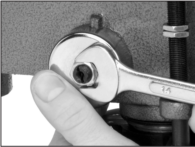
Figure 25. Loosening cover and jam nut
