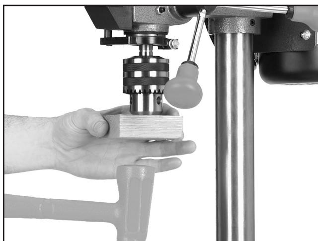
Figure 10. Seating the chuck on the spindle.
