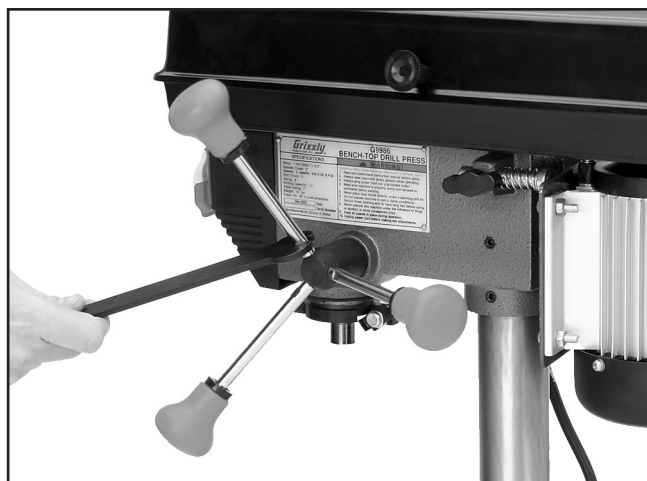
Figure 8. Tightening the downfeed handles.
