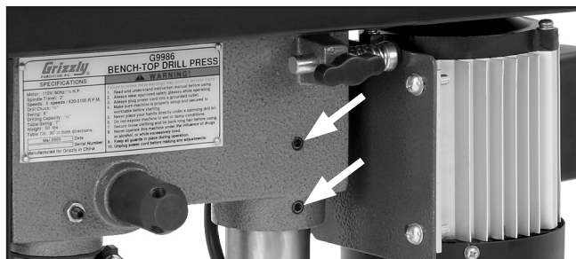
Figure 7. Setscrews for tightening headstock to column.
